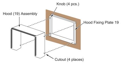
7. Press the top of the hood assembly to set the knobs in the cutouts.
